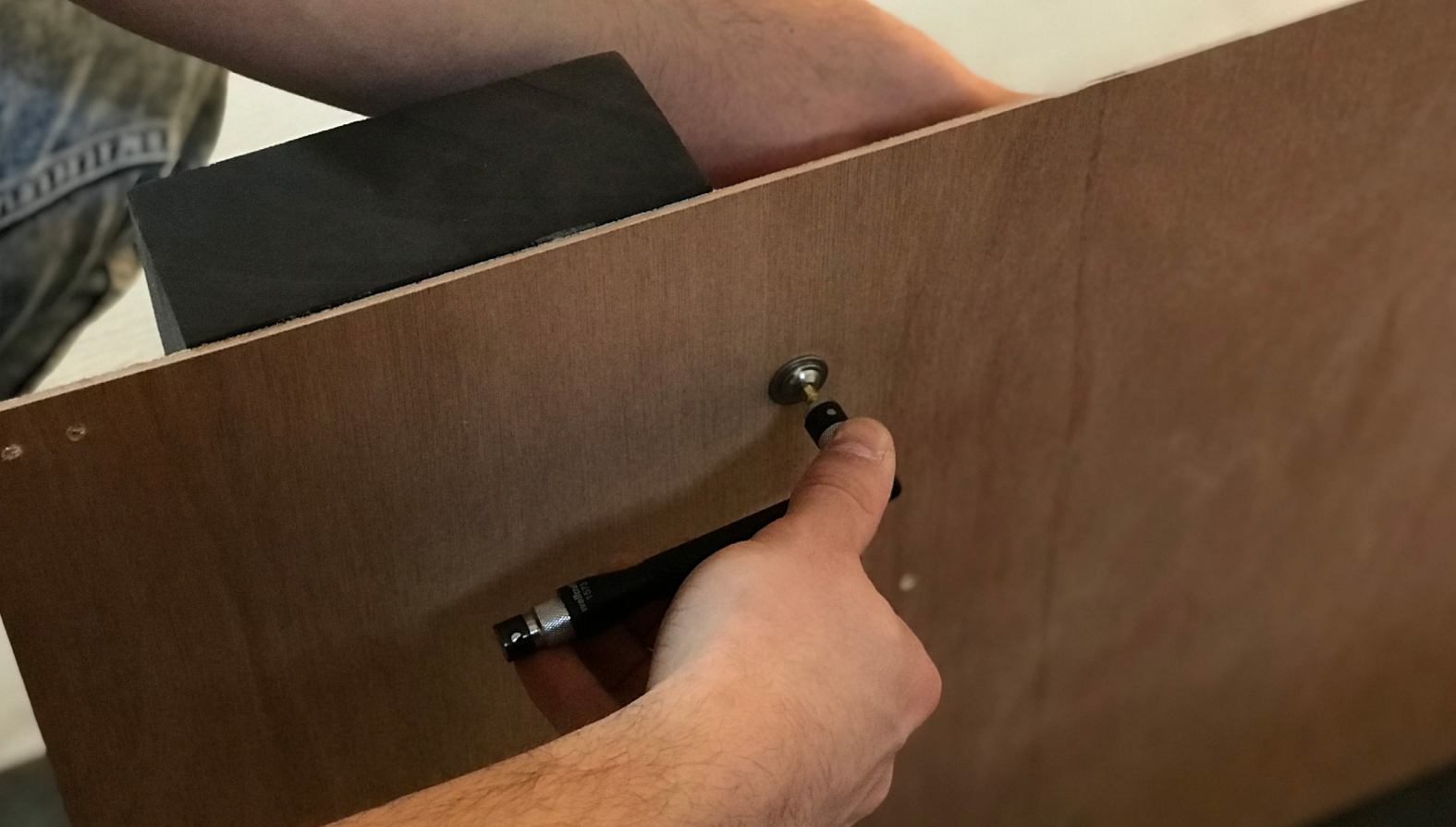
12. Keep holding the foot when unscrewing so it doesn't drop.
