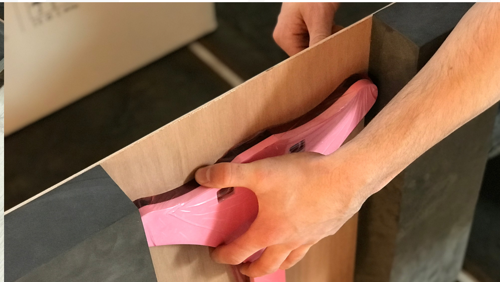
11. Fit the tool with the inside hex bit. Hold the foot firmly with one hand and use the tool in the other hand to unscrew the bolts.
