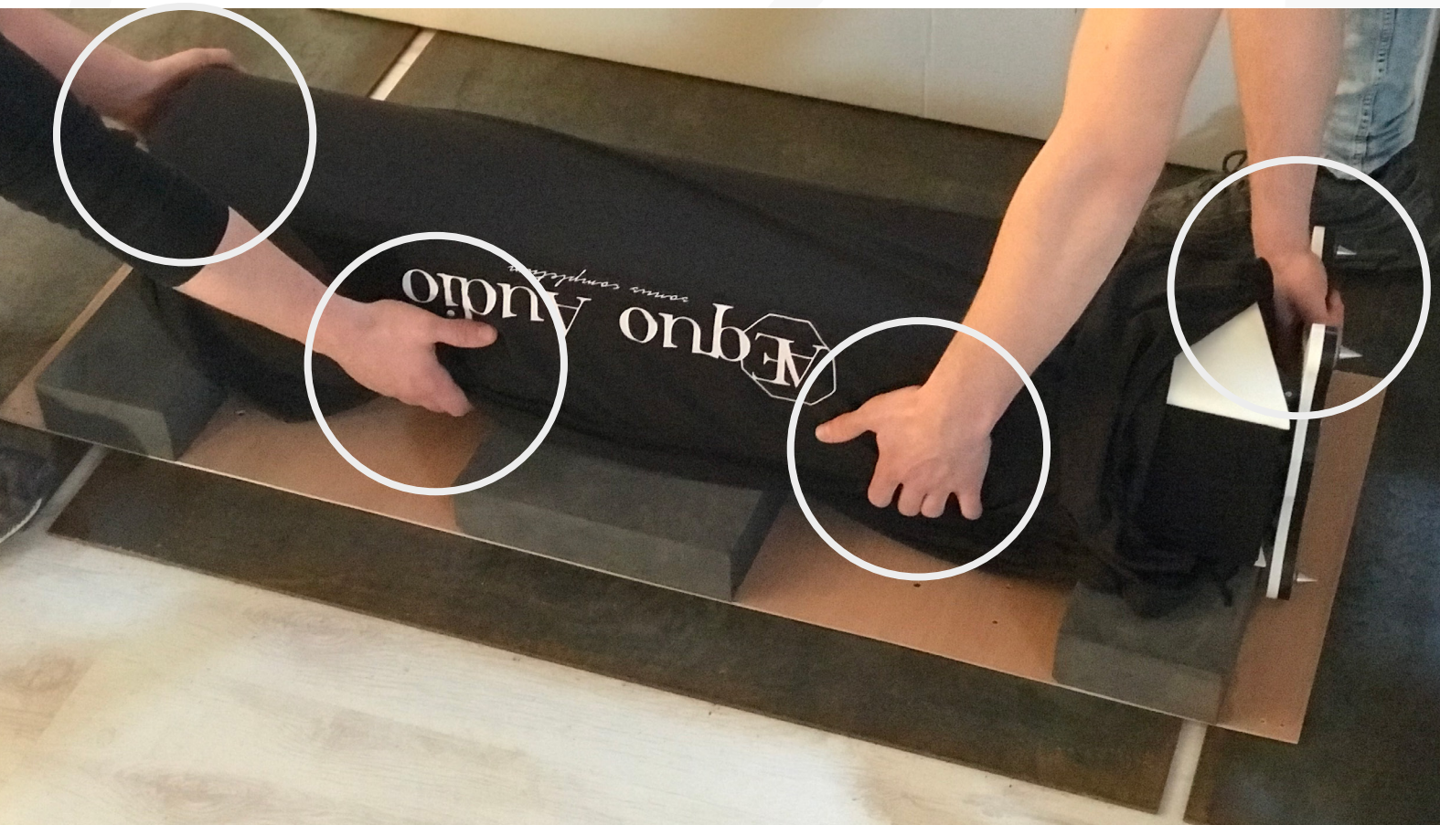
36. When lifting the Stilla, the positioning of the hand is very important.
