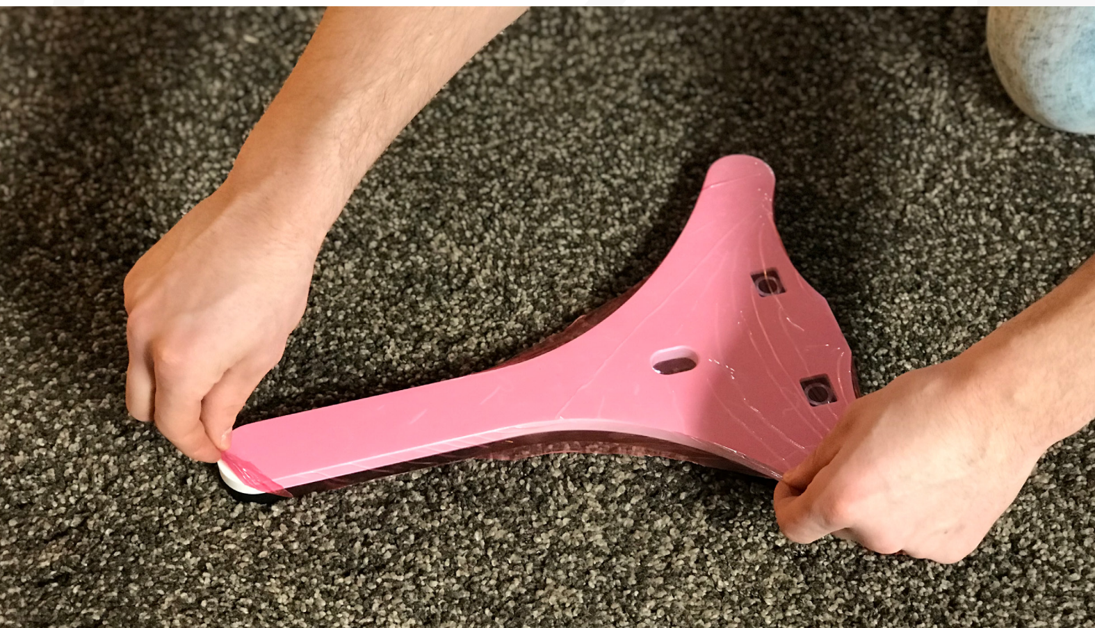
13. Place the foot on a soft surface. Find an edge on the protective foil and take it.
