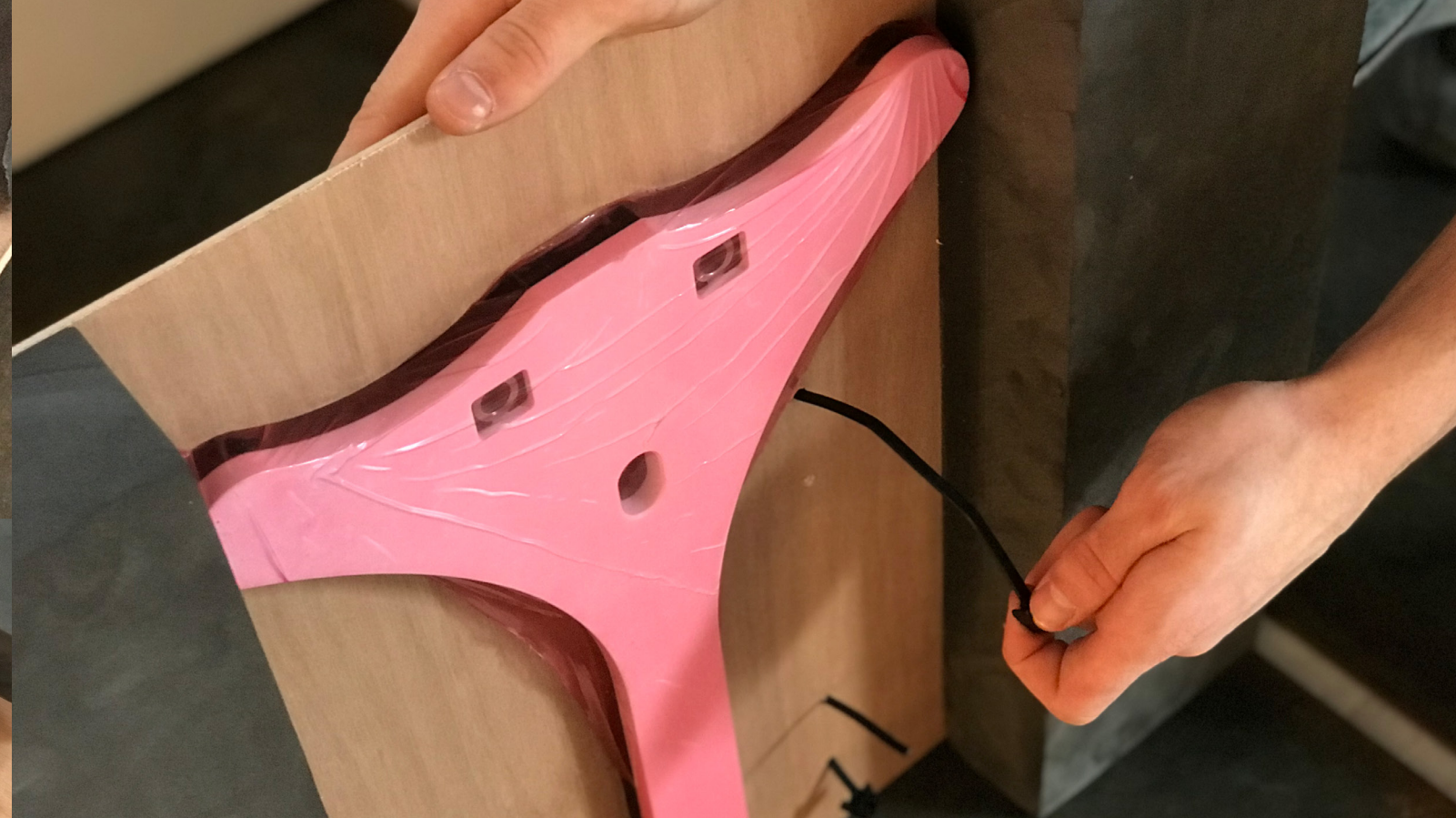
10. Place the board on its side and pull out the cable binders.
